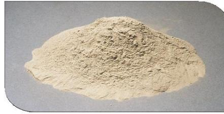
**Figure 1. Fly ash, powder resembling cement, has been used in concrete**
