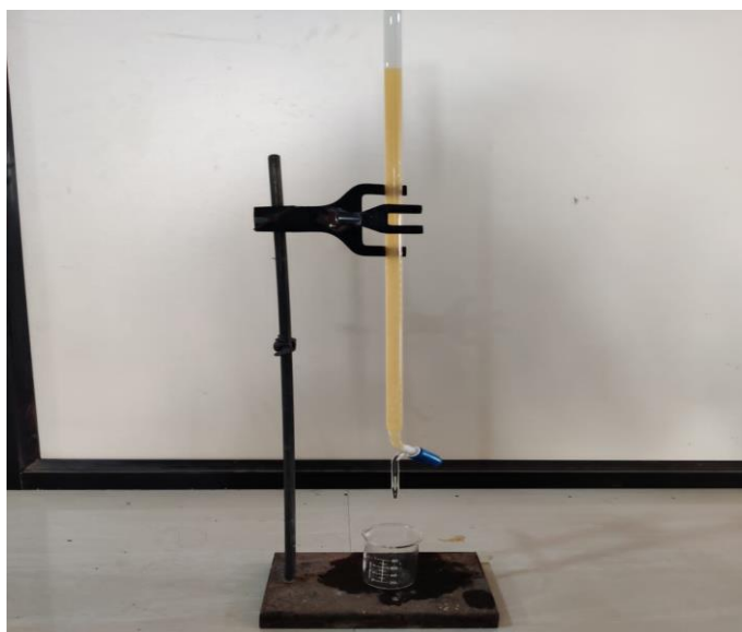
Fig No:4 Ion exchange Chromatography.
