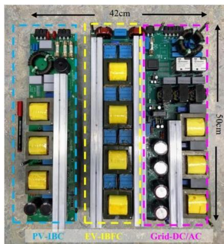
**Experimental 10kW three-port EV-PV converter prototype**
