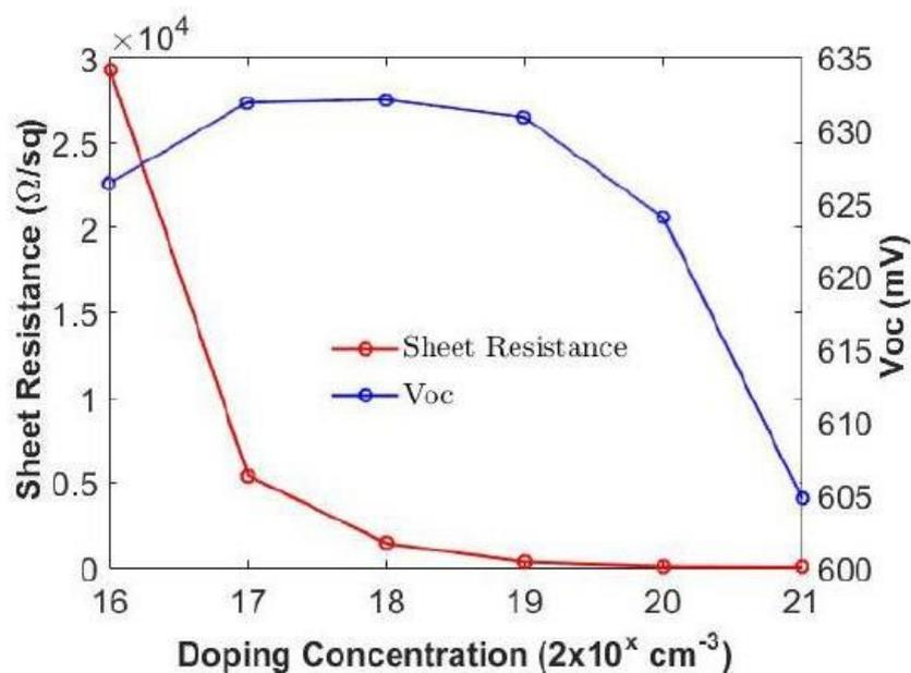
Because of its low sheet resistance, a device with a thickness of 150  $\mu\text{m}$  and an emitter doping concentration of  $2 \times 10^{20} \text{ cm}^{-3}$  was selected for this study. Both the sheet resistance and the overall performance of the device are significantly influenced by the thickness of the
