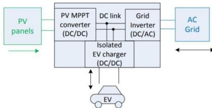
**Grid-connected, three-port, 10kW bidirectional EV-PV charger**
