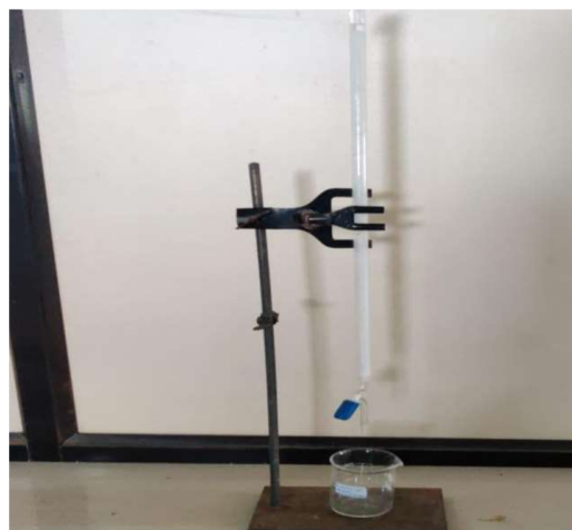
Fig No 3: Sephadex Gel Column Chromatography.
