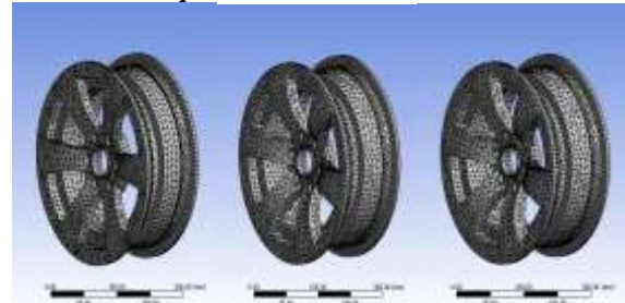
Fig: Meshing of different sizes of Alloy Wheel Model-1 (13X5J), Model-2 (13X5.5J), Model-3 (13X6J)
