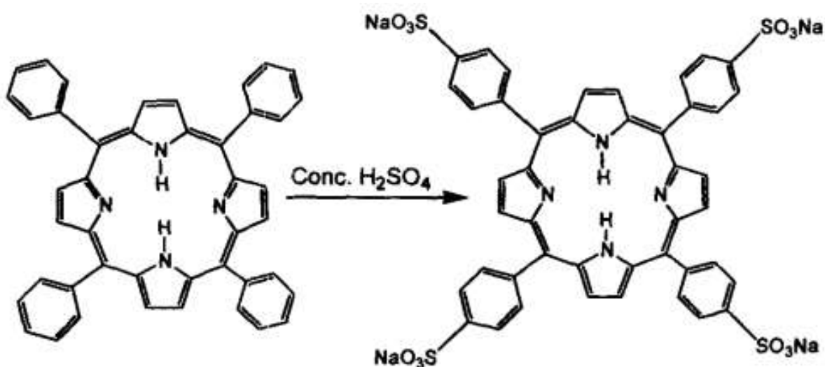
Figure 4: Sulphonation of The Tetraphenylporphyrin
