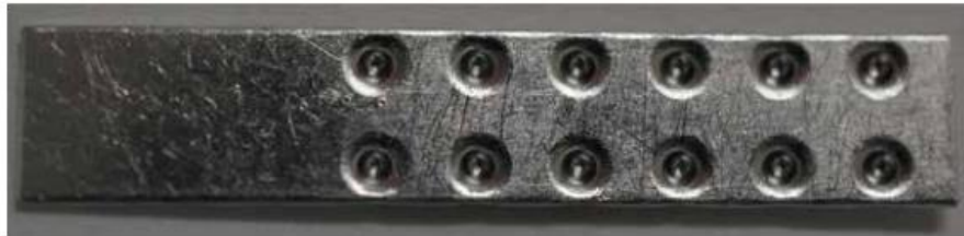
Size: 7 mm × 37 mm × 0.5 mm with ten wells (diameter 1.5 mm, depth 0.75 mm).
