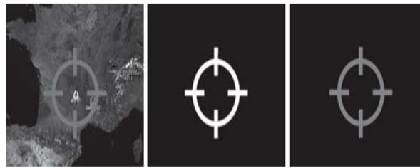
Figure: 1. From left to right, the first UI snapshot, the computed mask, and the final image after applying the mask are displayed.
