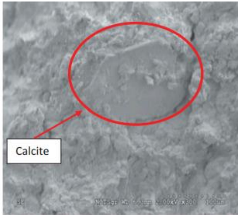
Figure 7 (c) Scanning electron micrograph of MICP treated dredged soil-1 O.D(7days-1.0M)
