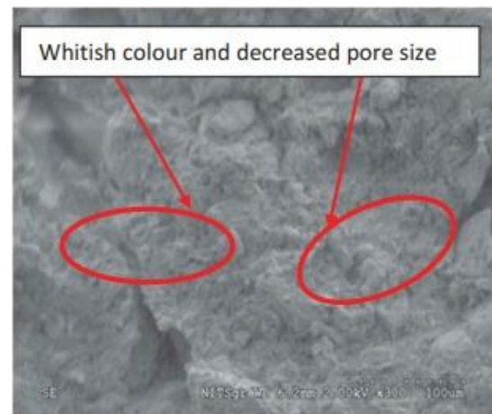
Figure 7(b) Scanning electron micrograph of MICP treated dredged soil-1.0 O.D (7days-0.25M)
