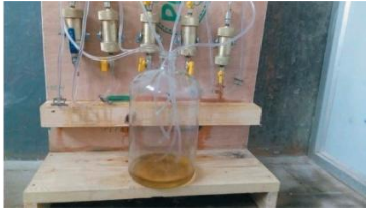
Figure 2: Treatment in process while as effluent gets collected for pH determination
